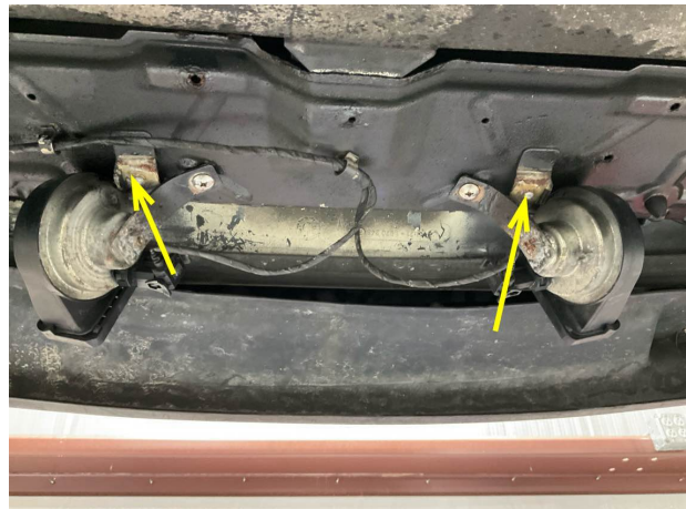
Original horn mounting points have bolts sheared
