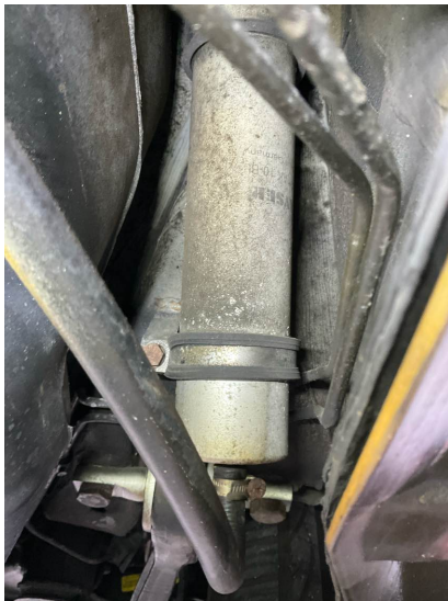
Fuel filter should probably be changed. It appears
