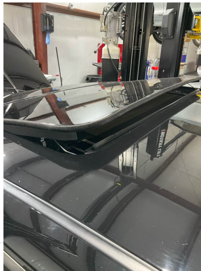
Sunroof failed in open position during testing. Will
