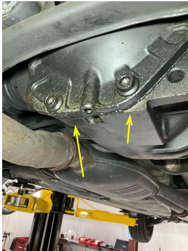
Seepage at differential
