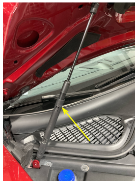
Hood struts weak at front hood
